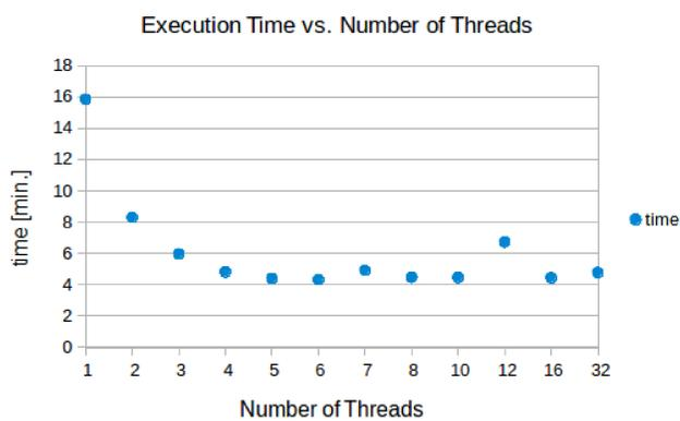
**Fig.3:** execution time with different numbers of threads. Calculating 32 points in z coordinate. Computed on a machine with Intel® Core™ i7-3770 Processor @ 3.40GHz with 4 cores and 8GB RAM.
