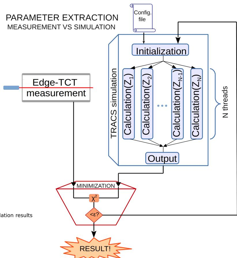
**Fig.4:** parameter extraction flowchart. Simulation results are fitted to measurements.
